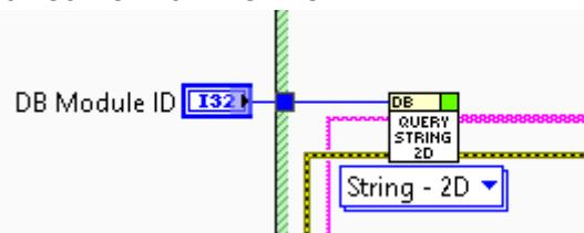
**5. Copy value from "Active Modules" to your SubVI "DB Module ID" front panel element and run.**
